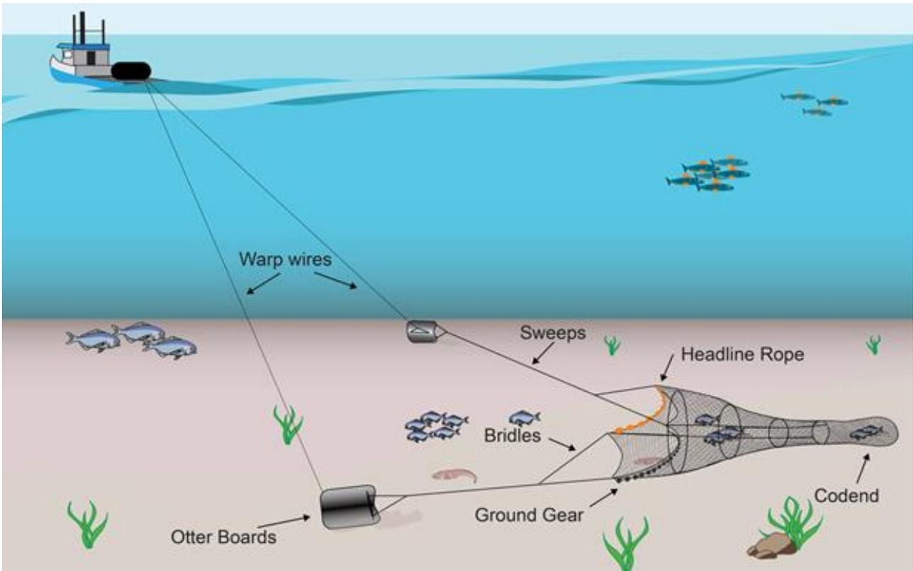
**Figure 7.** Schematic of a demersal trawl (Source: <https://www.afma.gov.au/fisheries-management/methods-and-gear/trawling>)
